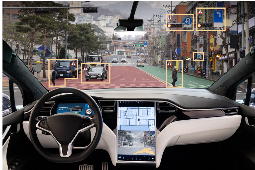
Figure 1.1: Illustration of the virtual vision of an autonomous car. Autonomous vehicles understand the surroundings with the help of cameras, sensors or radars. 1
