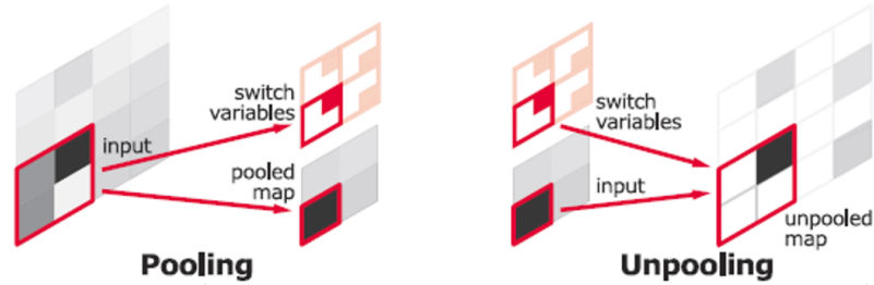
Figure 2.9: Illustration of pooling and unpooling in DeconvNet [35].
