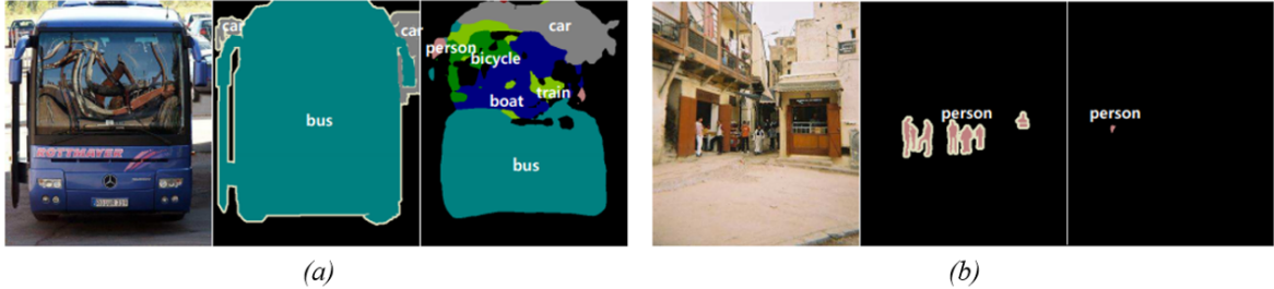
Figure 2.7: Instances of the drawbacks of FCNs model [35]. (a) Too large objects face over segmentation issue; (b) Too small objects is missed.
